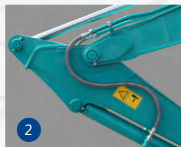
layout of pipe on the working device beautiful—high reliability Pipeline layout more reasonable, reduce the probability of wear. The hydraulic hose had passed 1000000 time pulse test, improved hose reliability. Strengthen the work device, The durability has passed the FEM and long term durability test.
