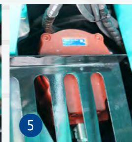
Swing motor gear box lubricated by hydraulic oil, not need to change the lubrication oil
